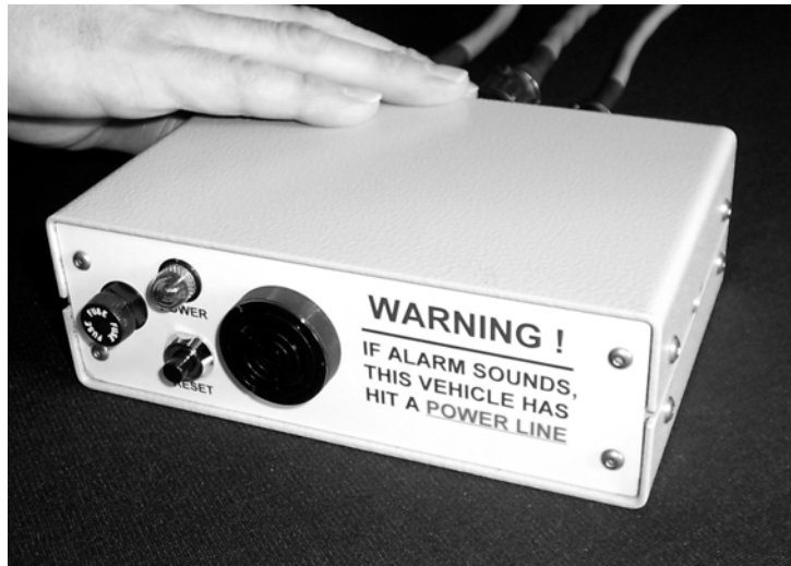
Figure 11 Control module for the prototype power line contact alarm system.
